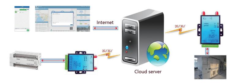
GT90 Embedded Modbus RTU serial port server function, even in the absence of a network, it can still automatically complete data acquisition and storage.
