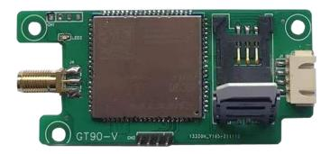
When using a SIM card, please first pay attention to the **OPEN** and **LOCK** words and directions on the SIM card holder. As shown in the picture, gently press and hold the card cover and slide it down to open the SIM card holder; press and hold the card cover and gently slide it up to close it. Tighten the SIM card holder.
