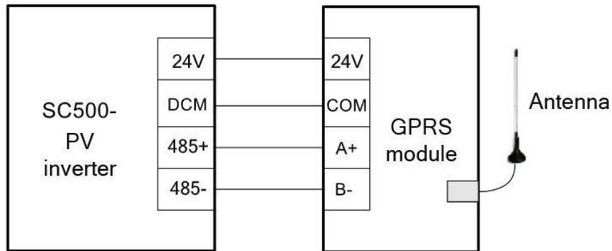
Connection between the GPRS module and the inverter
