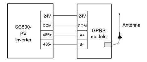
Connection between the GPRS module and the inverter
